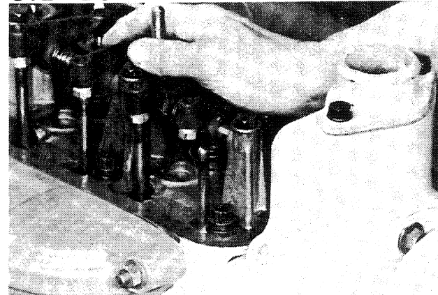
Release rocker arm assembly and position push rod beneath rocker arm adjusting screw.
