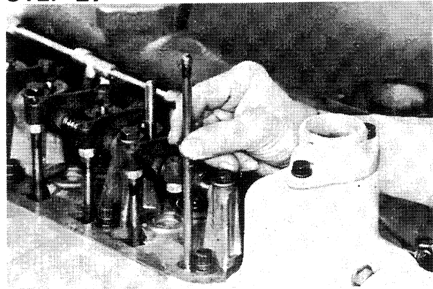
Install the push rod.
