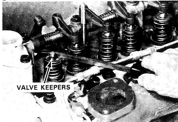
Keeping the valve spring compressed, install the valve keepers in the upper valve stem groove. Remove screwdriver and tap end of valve stem to seat keepers.
