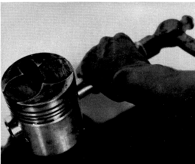
Figure 17 Removing Piston Pin
