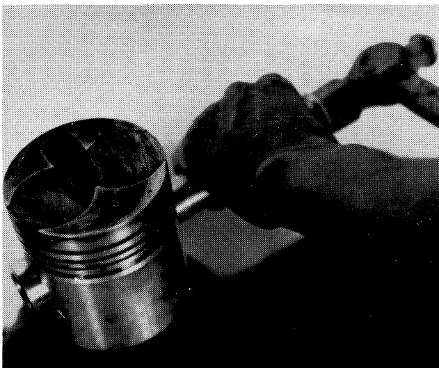
Figure 17 Removing Piston Pin
