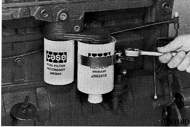
Use a strap wrench to remove the fuel filters.
