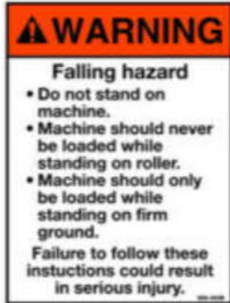
Fig. 2 - Safety decals - implement; replace immediately if damaged.
