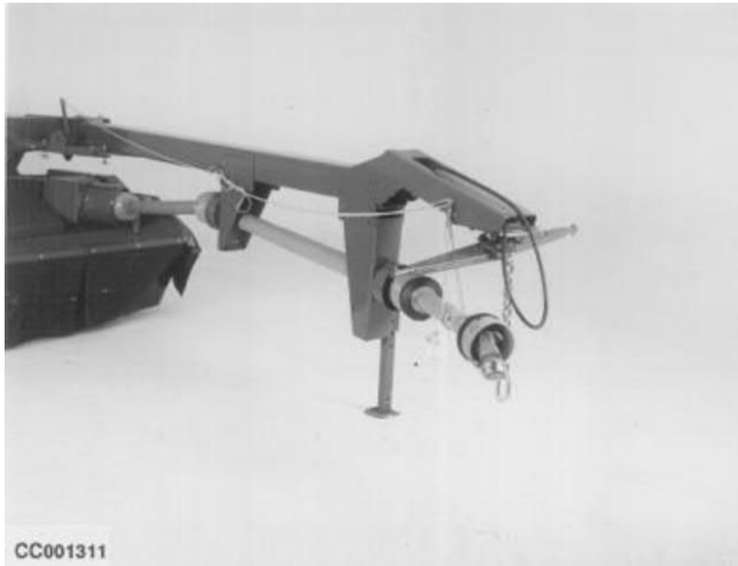
Version with linkage drawbar tongue
