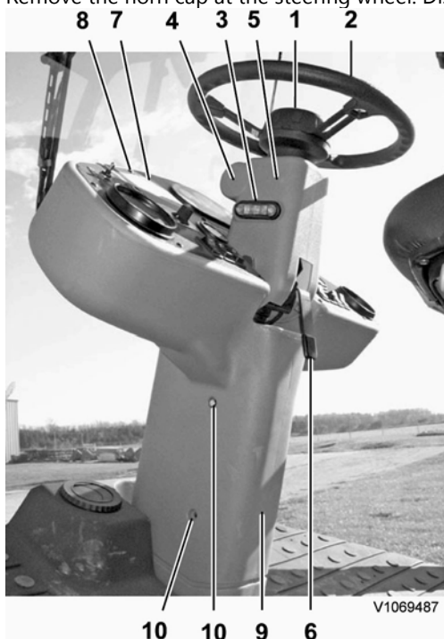
Figure 1 Steering column components
