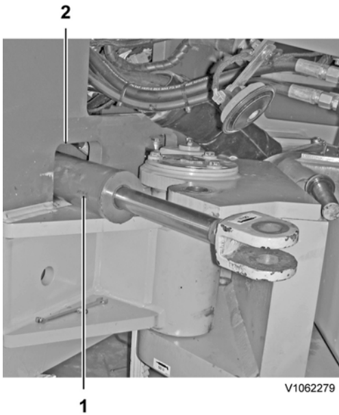
Figure 4 Cylinder removing from frame opening
