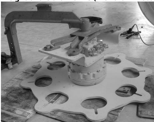
Figure 1 Tool assembled to drum drive assembly
