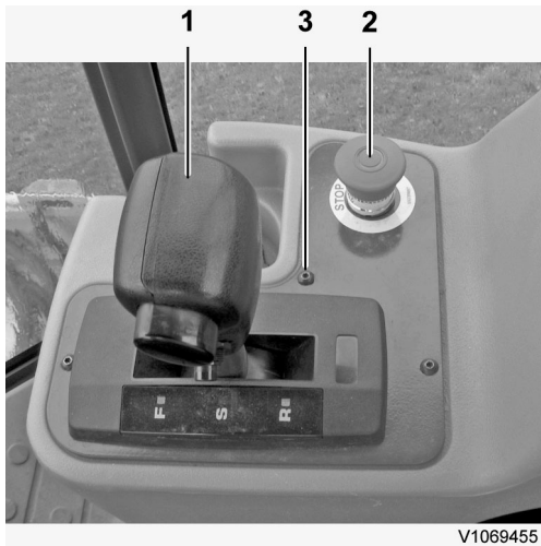
Figure 3 Hydrostatic controller at the side console
