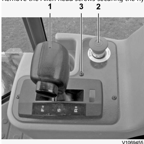
Figure 1 Hydrostatic controller at the side console
