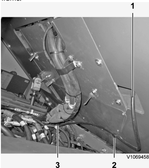
Figure 2 Controller cable routing below the operator's platform
