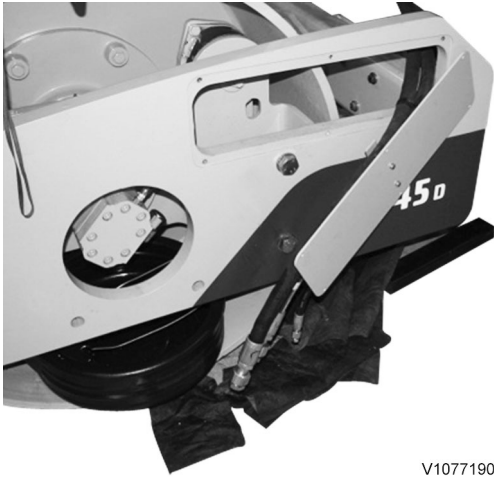
Figure 2 Hose cover plate removed with hoses attached
