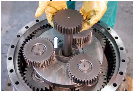
Figure 5 Removal, 1st stage sun gear
