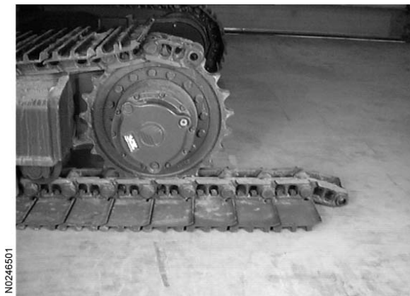
Figure 7 Fitting of track
