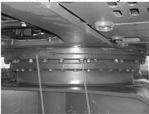
Figure 5 Removal, superstructure mounting screws
