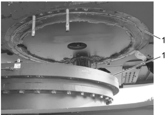
Figure 3 Clean the mounting surface
