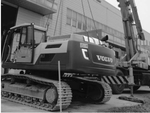
Figure 6 Removal, lifting superstructure (1)
