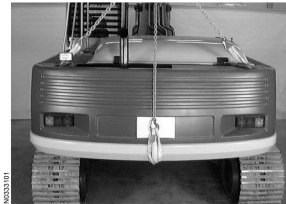
Figure 9 Ready for lift
