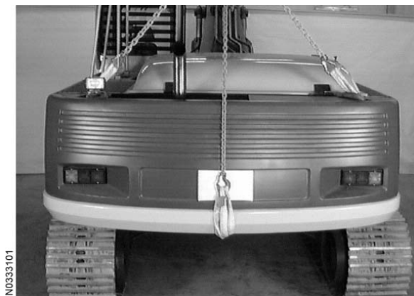
Figure 4 Lifting tools fitted
