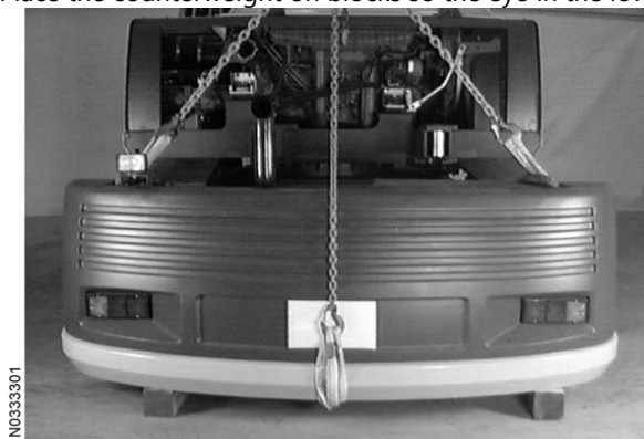
Figure 10 Counterweight lifted away
