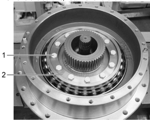
Figure 6 Removal, screws (1) and retainer (2)
