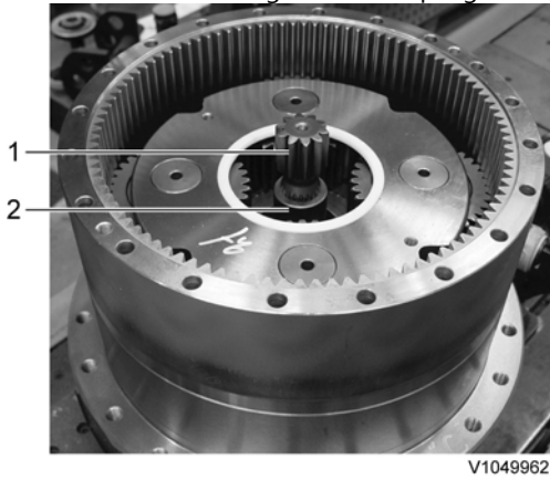
Figure 3 Removal, No.1 sun gear (1) and coupling (2)
