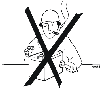
Figure 2 Do not smoke near batteries!
