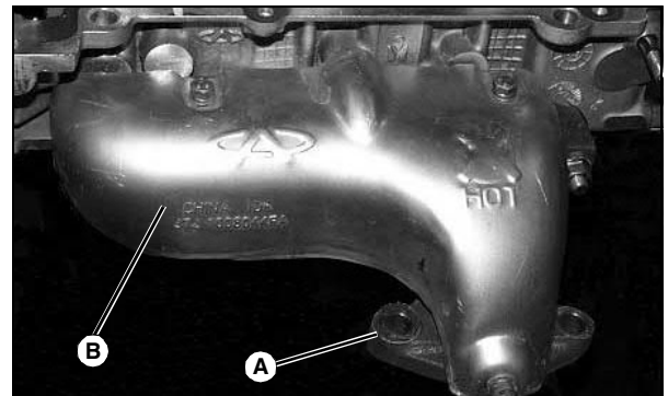
a. Exhaust manifold (A) and shield (B), muffler pipes (C), muffler (D) and muffler shield (E).
