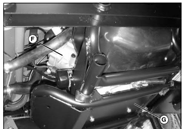
c. Between engine (F) and skid plate (G) (if equipped).
