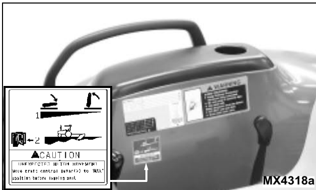
Picture Note: Label installed on tractors equipped with optional draft sensing kit.
