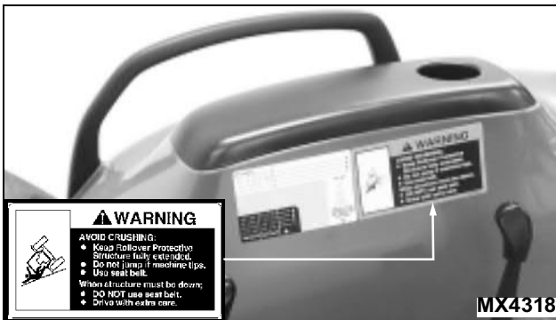
Picture Note: Label attached to right fender when tractor is equipped with a folding ROPS
