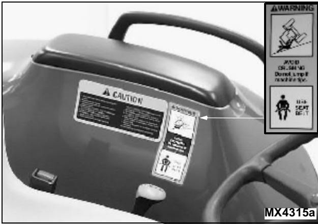
Picture Note: Label attached to left fender when tractor is equipped with a fixed ROPS
