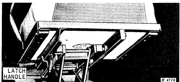
Seat Tipped Up (Orchard Tractors with Rockshaft)
