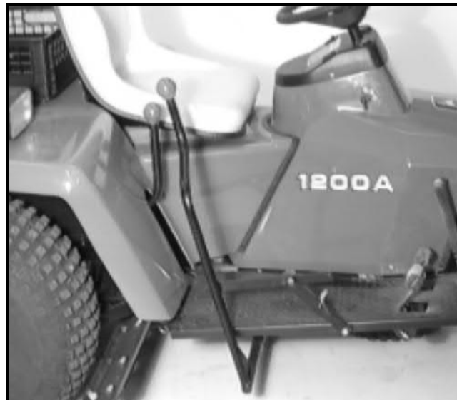
K - Cultivator Handle .....Lowers and raises cultivator.
