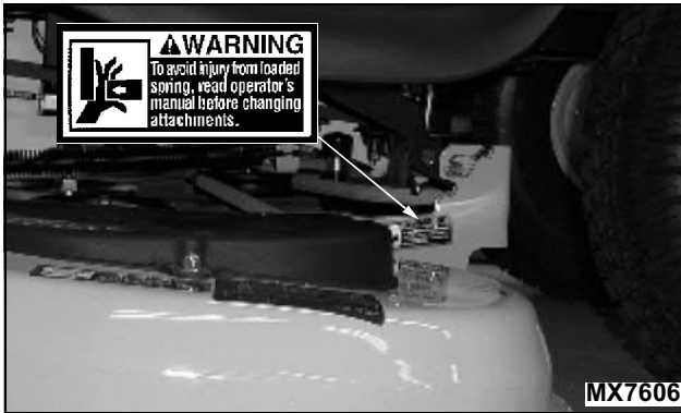
Picture Note: Two decals, one on each mower deck lift bracket. 48C shown.
