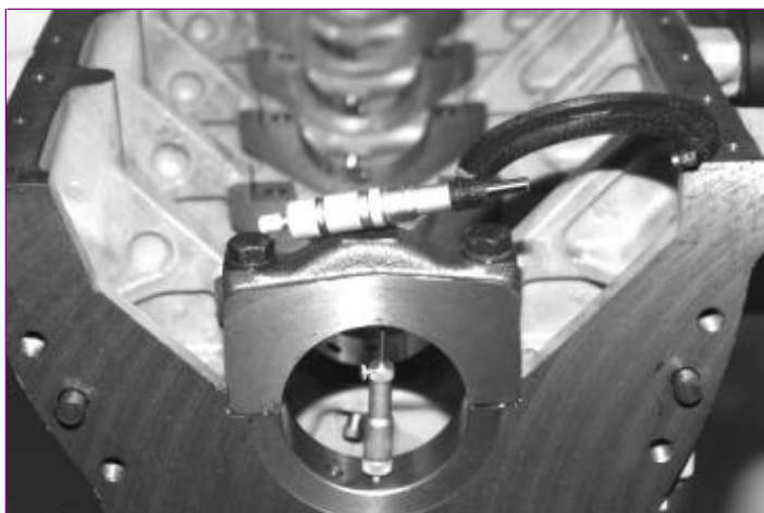
RG7537-UN: Measuring Assembled Main Bearing Cap ID
