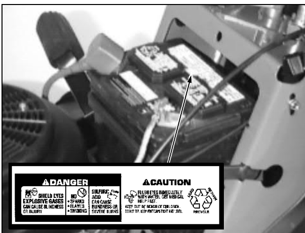
Picture Note: Label is located on battery
