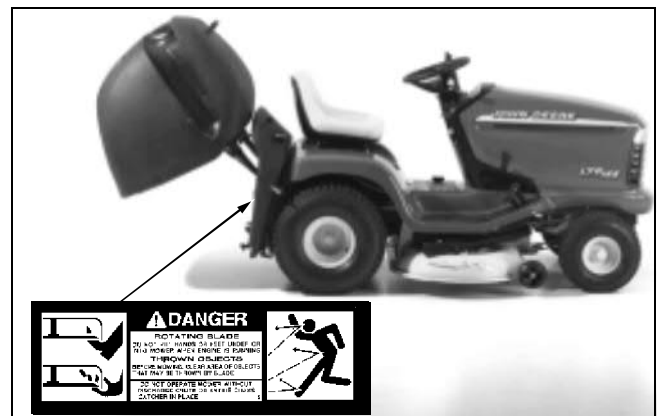
Picture Note: Decal is located to the right of discharge chute opening.
