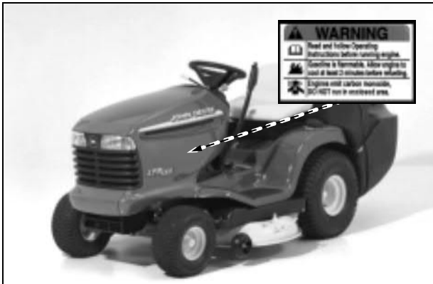
Picture Note: Label is located on Left-Hand Side of Briggs and Stratton Engine
