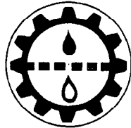
Fig. 6-Transmission Oil Filter Indicator Light
