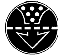
Fig. 8-Air Filter Indicator Light
