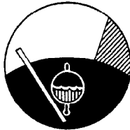
Fig. 12-Engine Coolant Temperature Gauge
