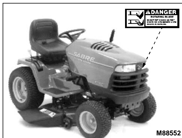
Picture Note: Located on Left-Hand side of deck
