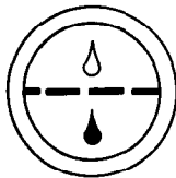
Fig. 36-Hydraulic Filter Restriction Indicator Light
