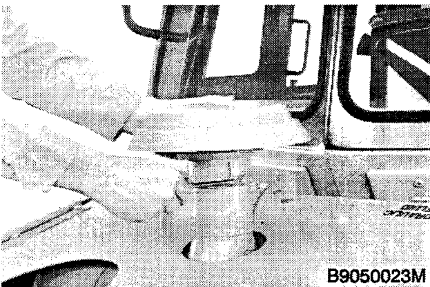
Loosen the clamp and remove the cap for the air cleaner. If the air cleaner is equipped with a precleaner, remove the precleaner.
