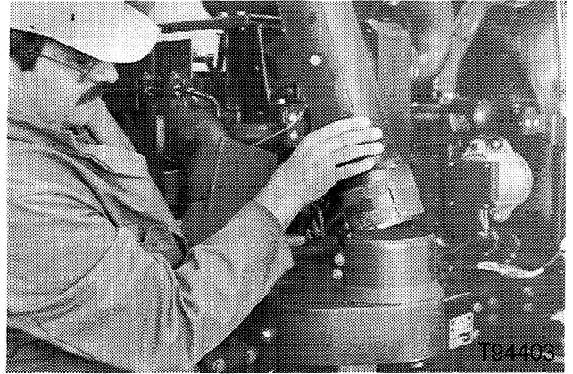
Remove the exhaust pipe.
