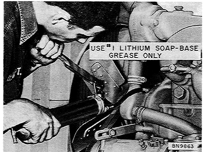
Figure 8 - Lubricating Fan Shaft Bearing
