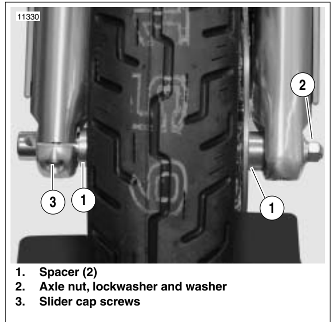
Figure 2-7. Front Axle Assembly
