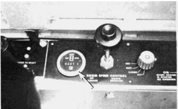
Electric Service Meter
