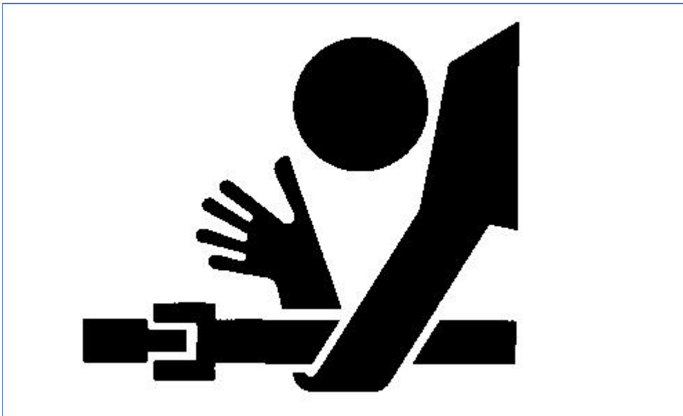
TS276-UN: Beware of rotating PTO shafts
