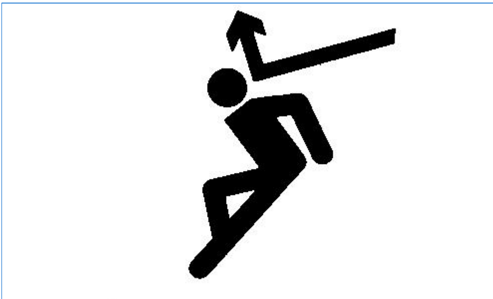
TS263-UN: Cable Recoiling
