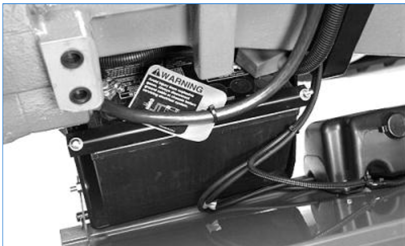
RW56299-UN: Avoid Explosive Gases Decal Location
