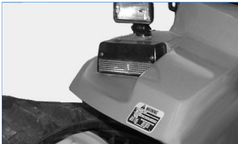
RW26419-UN: Stay Clear of PTO Decal Location
