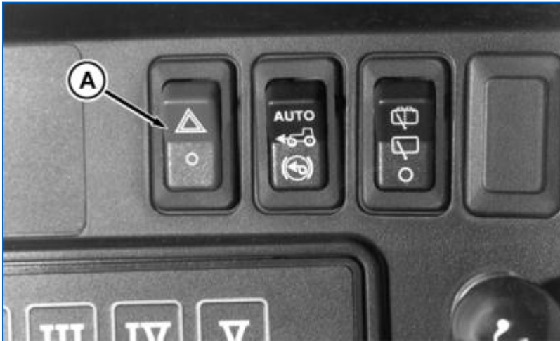
RW26650-UN: Push Switch to Activate Lights
