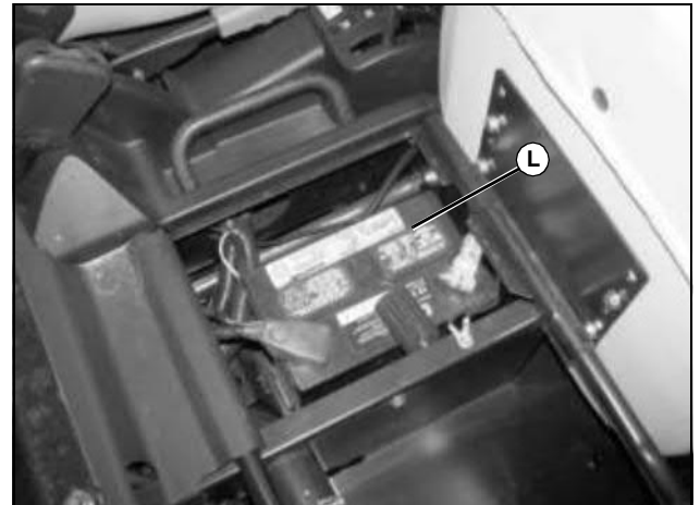
e. Battery (L) and related wiring harnesses.
