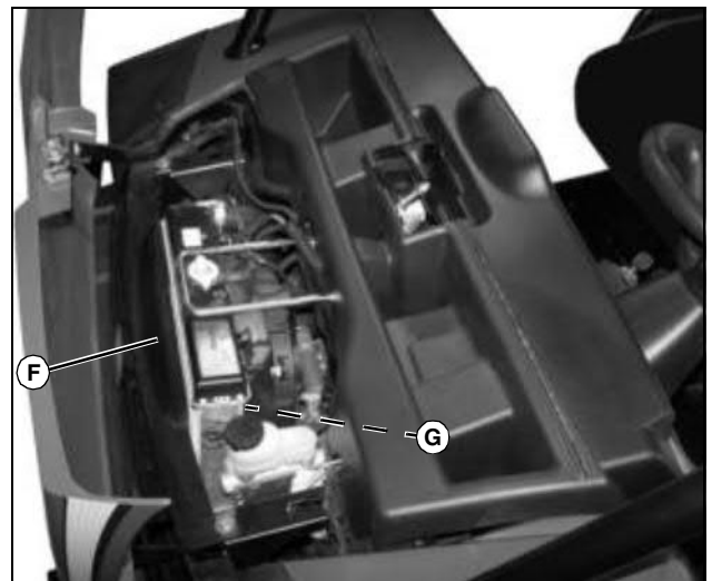
b. Intake screen (F), and radiator cooling fins (G).
