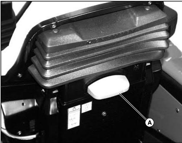
A - Seat Height Adjustment Lever
