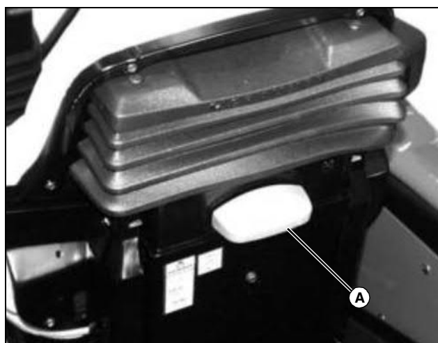
A - Seat Height Adjustment Lever
