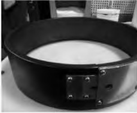
Illustration 13 g03150408 Old laminated phenolic (rawhide) tool - Front side of tool
