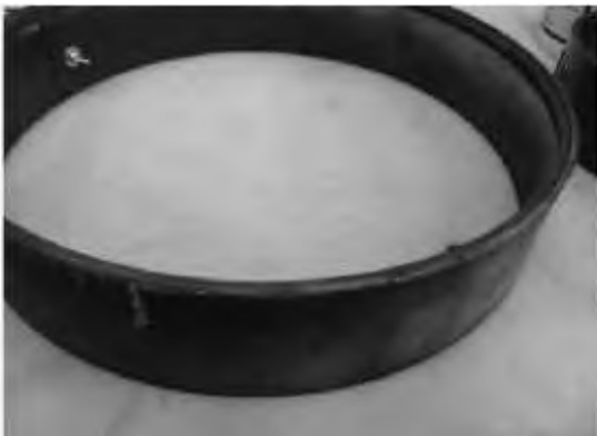
Illustration 14 g03150409 Old laminated phenolic (rawhide) tool - Back side of tool
