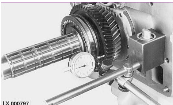
LX000797-UN: Check Gear Axial Play
