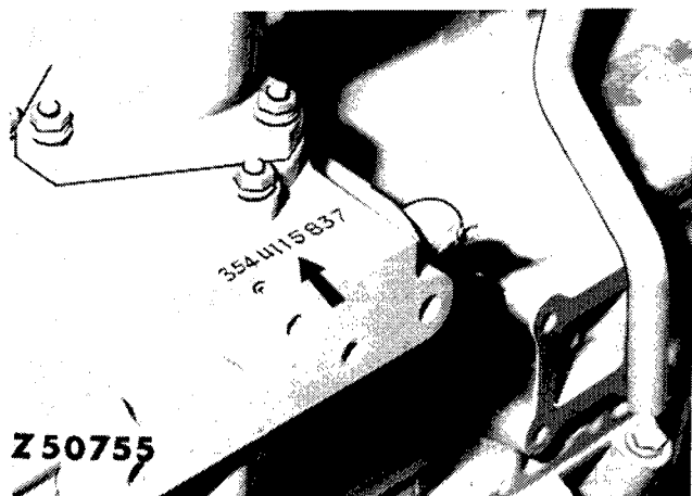
Fig. 4 — Serial Number Stamped into Perkins Engine
