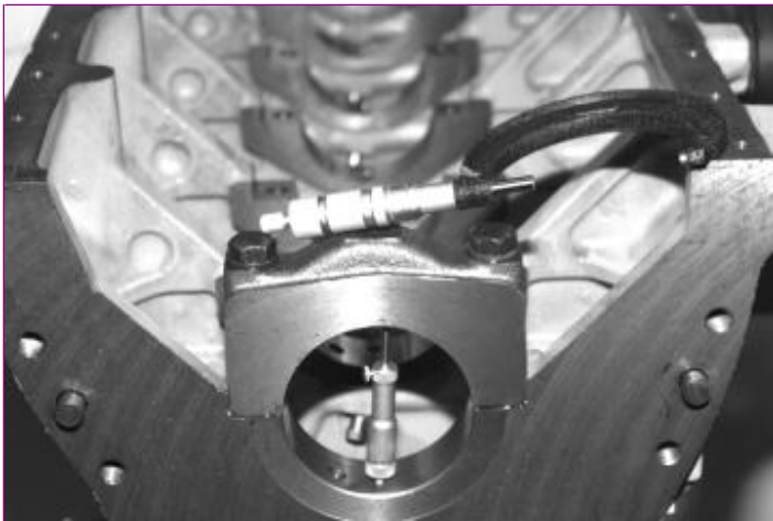
RG7537-UN: Measuring Assembled Main Bearing Cap ID
