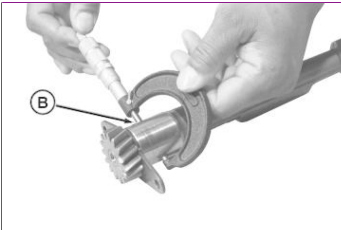
RG17354-UN: Balancer Shaft Journal OD Measurement
