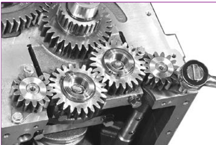
RG13039-UN: Balancer Shaft Removal
