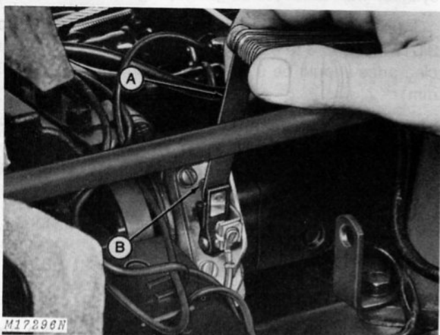
A—Flat Feeler Gauge B—Gap Adjusting Screw
