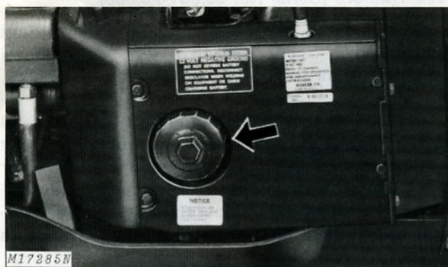
Fig. 3-Changing Engine Oil Filter
