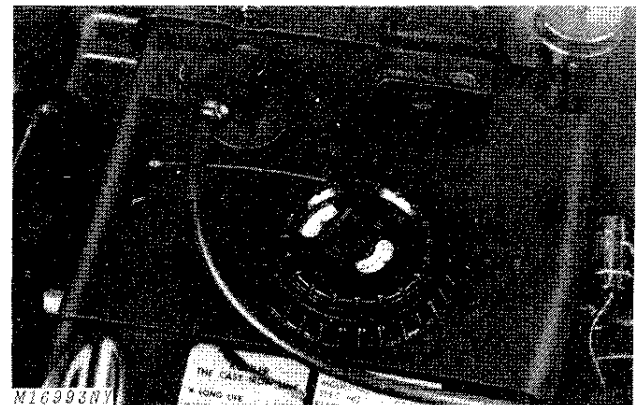
Fig. 12-Checking Engine Speed With Vibration Tachometer
