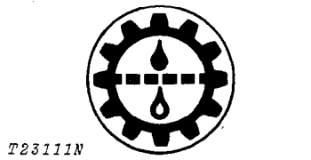
Fig. 29-Transmission Oil Filter Indicator Light
