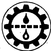
Fig. 80-Transmission Oil Filter Indicator Light
