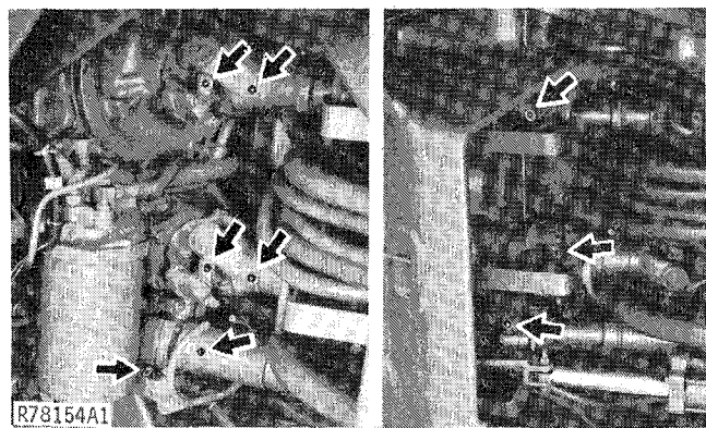
Fig. 9-Hinge Area Grease Fittings (Front and Rear)
