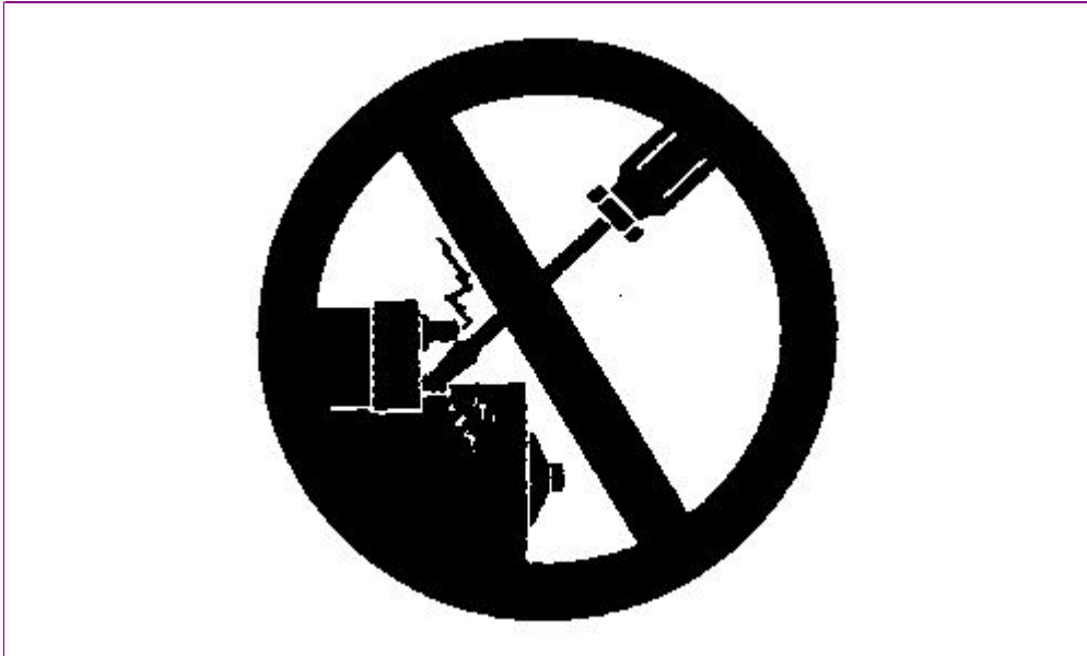
RG5419-UN: Prevent Bypass Starting
