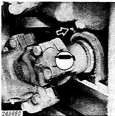
Fig. 18-Lower Drive Shaft Support Bearing (1 Point)
