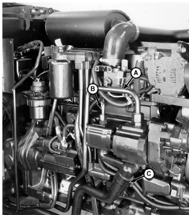
A—Hydraulic Pump-to-Inlet Housing Line B—Hydraulic Pump-to-Steering Valve Line C—Suction Line
